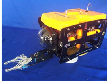
Figura 2: Robot submarino ROV110
