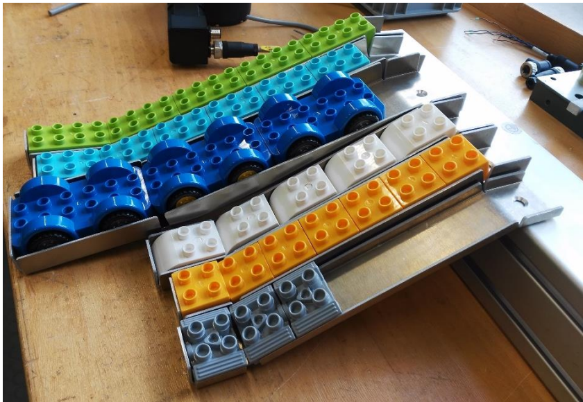
Figure 3-1 Manufactured Slides for the Assembly Station
