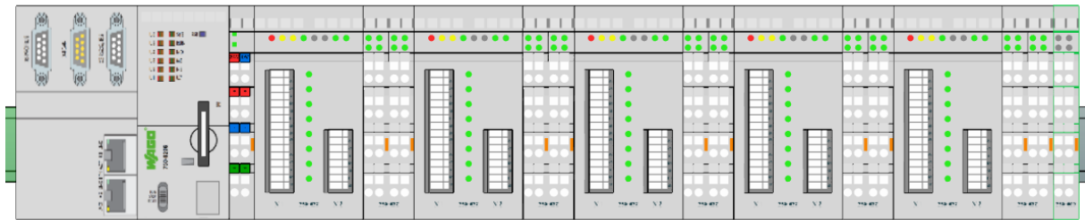
Figure 2-29 Set-up of the 5DOF Robot's PLC
