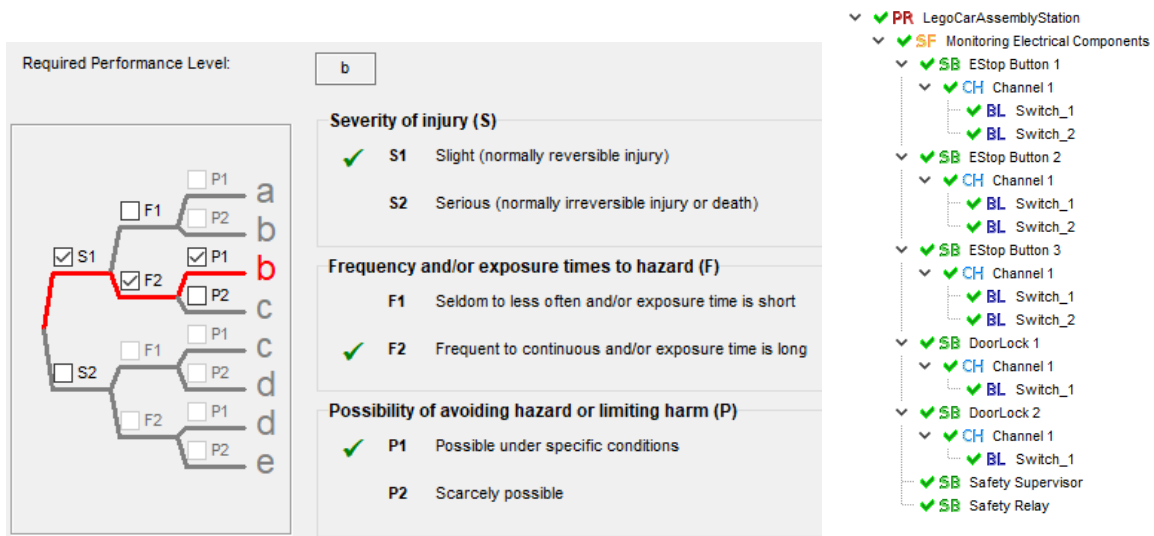
Figure 3-12 Definition of the Performance Level of the Safety System
