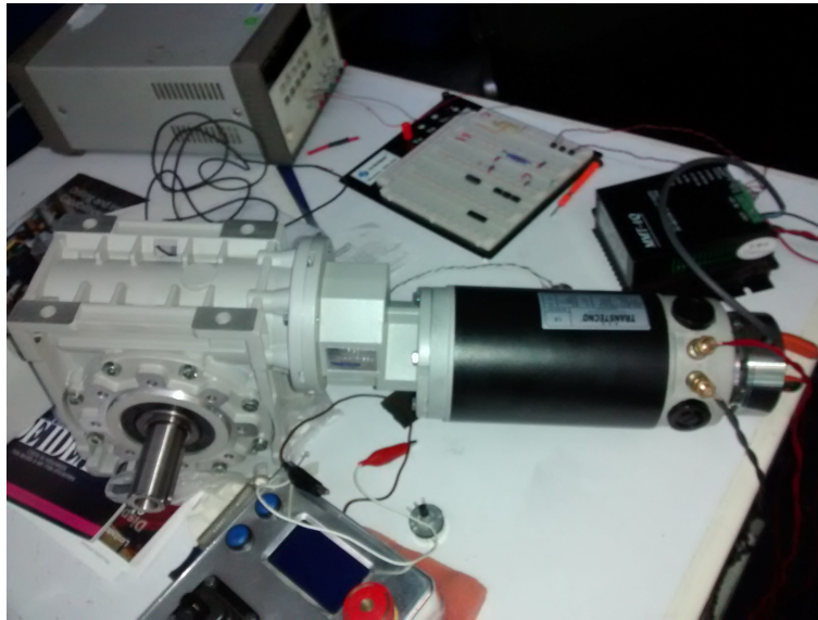
Figura 3.1.4: Motor-reductor TRANSTECNO EC600.240BR.
