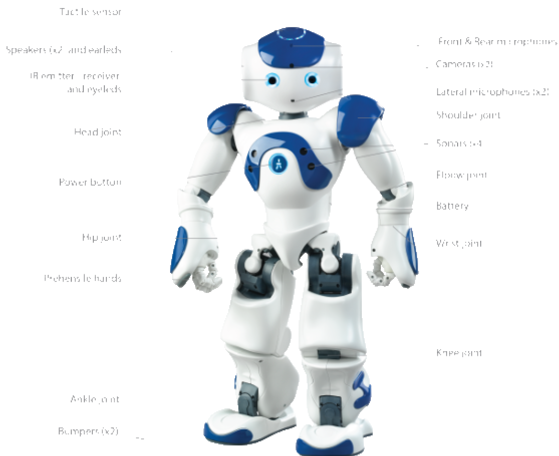
Sensors and Actuator of the humanoid robot NAO
