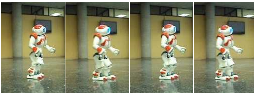
Figure 4.9 - Images of the implementation of a straight line backwards walking pattern
