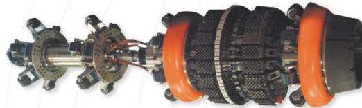
Figura 18: Diablo instrumentado, BJ Pipeline Inspection Services
