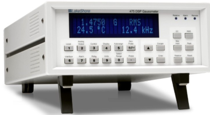
Figure 4.4: Gaussmeter used to measure the magnetic field
