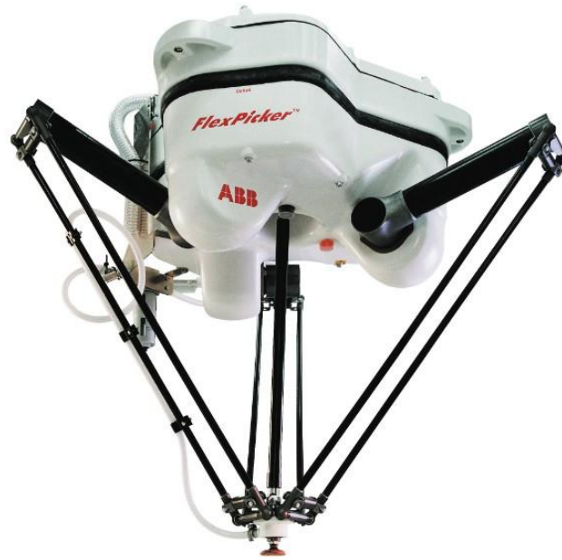
Figure 2 Example of an ABB IRB 340 delta robot. Image from [7].
