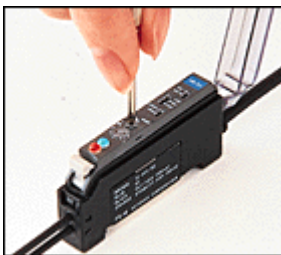
Image 4.2 FSM1 Fiber sensor[5]
