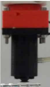
Image 3.2 End effector in delta robot
