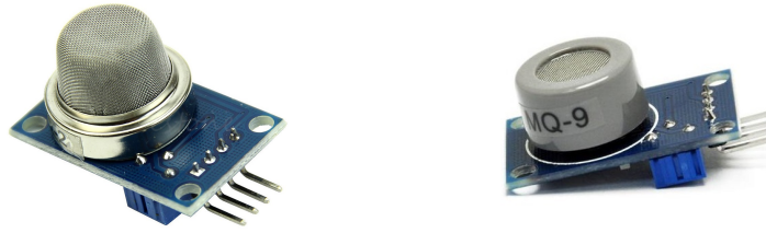
(a) MQ2 toxic and flammable gases sensor and module. (b) MQ9 toxic and flammable gases sensor and module.
