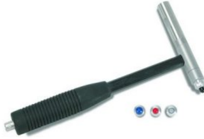
Figure 7.4: 086C40 Impact Hammer used to excite the Building-like structure and its different tips, taken from [28].
