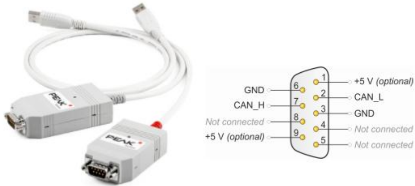
Figure 17. Pin assignment of PCAN-USB [15].
