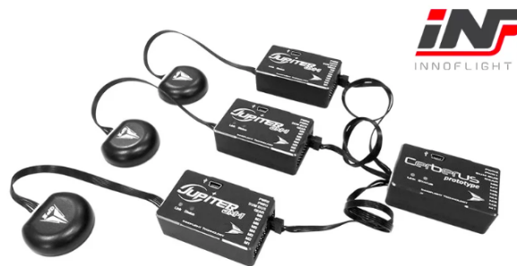
Figure 2.3: Cerberus triple redundant autopilot, taken from [6]
