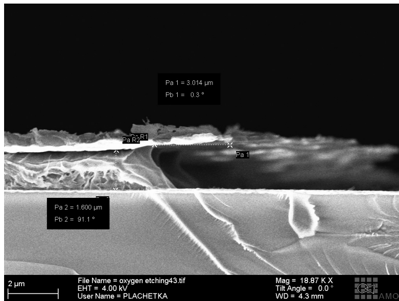
Figure 6.20: Etching of PVDF through oxygen etching
