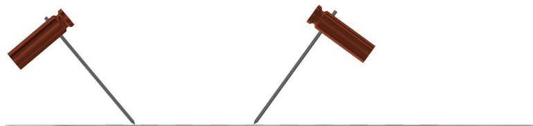
Figure 6.25: The image shows the probes getting in contact with the metal conductive pads of the fabricated capacitors created over the surface of a wafer
