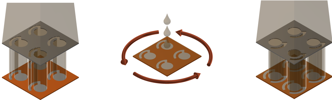
Figure 7.1: Fabrication process for sensor, the electrodes are fabricated through shadow masked sputtering, the PVDF-TrFE active layer is cast through spin-coating techniques and a last electrode is sputtered
