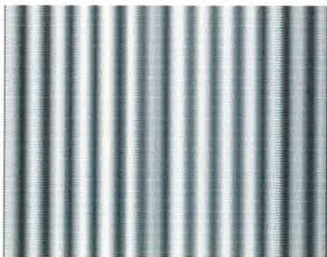
Fig. 4. Fringe Pattern projected on a reference plane
