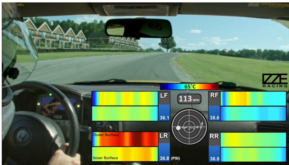
Figure 3-16: Driving test made by the own company Izzе Racing, with the “tire temperature sensor” (Outer Surface) & the “Tire Temperature & Pressure Monitoring System (TTPMS)” (Inner Surface) simultaneously [IR18b]
