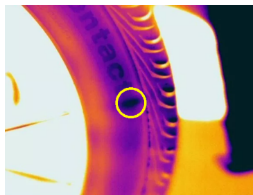
(b) Detection of a bubble caused by delamination in the sidewall of the tire [IIS18]
